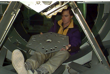
Peter Tuthill with an aperture mask for the 10 m Keck telescope
